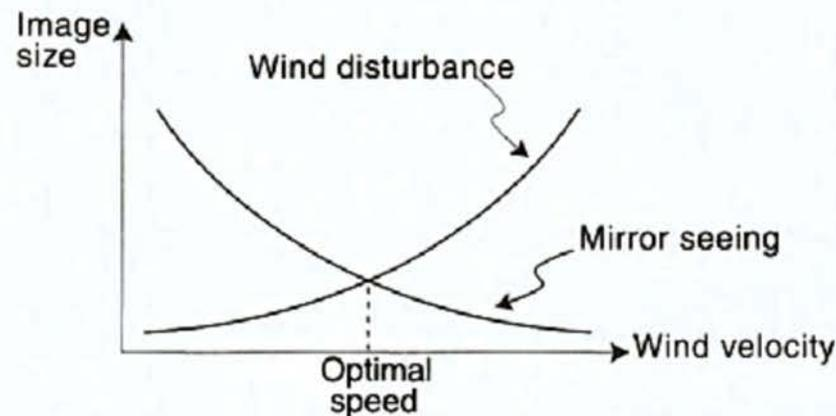
**Fig. 9.10.** Notional plot showing how mirror seeing improves with wind velocity while dynamic effects worsen. Optimal wind speed can be maintained by adjusting the enclosure’s louvers and windscreen.
