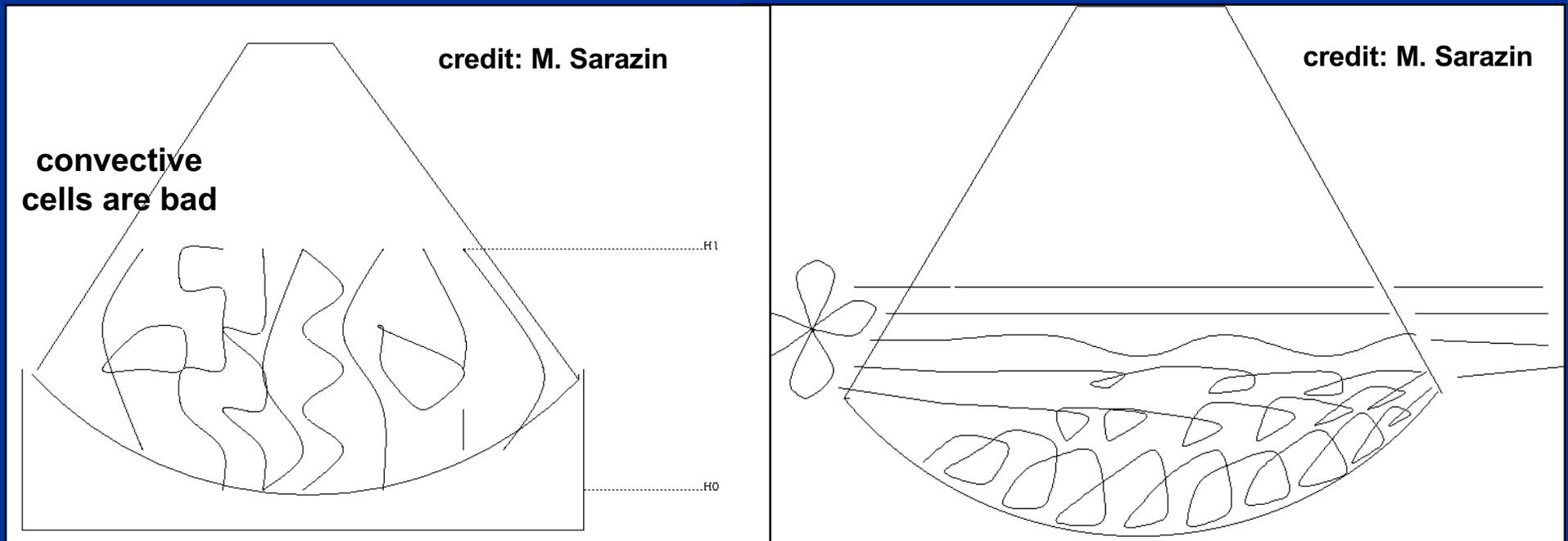
To control mirror temperature: dome air conditioning (day), blow air on back (night), send electric current through front Al surface-layer to equalize temperature between front and back of mirror
